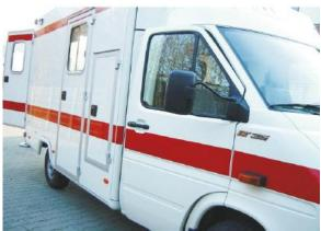
**RESCUE III (EMERGENCY RESCUE VEHICLE)** is the largest and most spacious model. With a height of up to 1.97m the interior provides plenty of headroom. The vehicle platform for this model is a **Volkswagen chassies or Mercedes Benz Sprinter box chassies**, with a van structure added. This is of aluminium sandwich sheet / construction.
